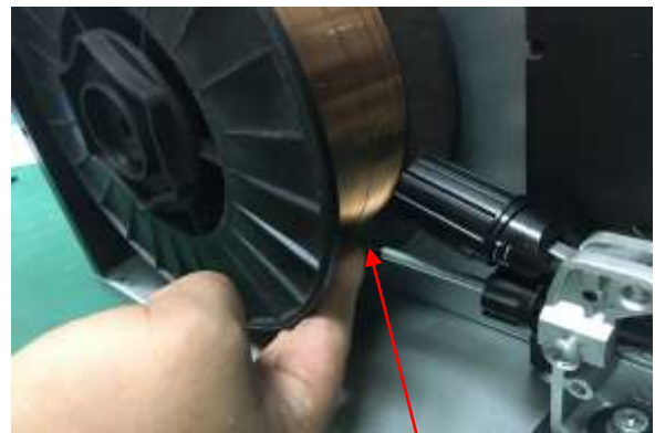
(4) Snip the wire carefully, be sure to hold the wire to prevent the spool uncoiling. Carefully feed the wire into the inlet guide tube of the wire feed unit.
