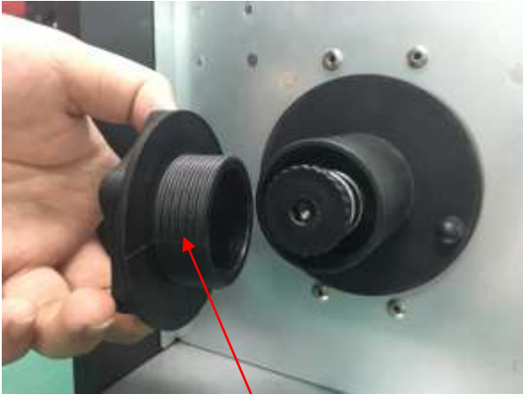
(1) Remove the spool retaining nut.
