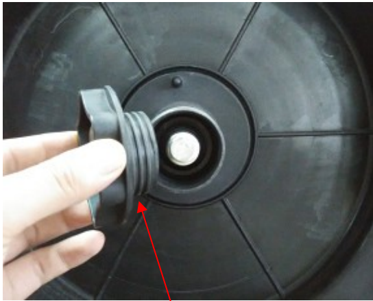
(1) Remove the spool retaining nut.
