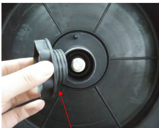
(1) Remove the spool retaining nut.
